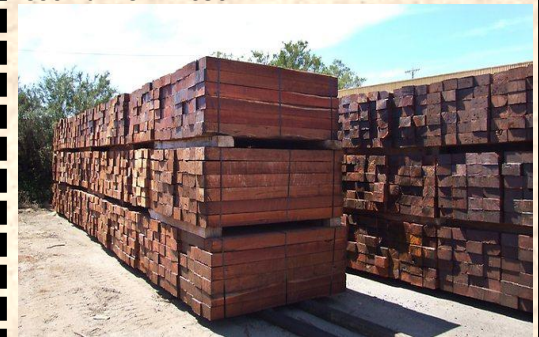
The sleepers needed to get Cooma Monaro Railway Inc. back on track.
